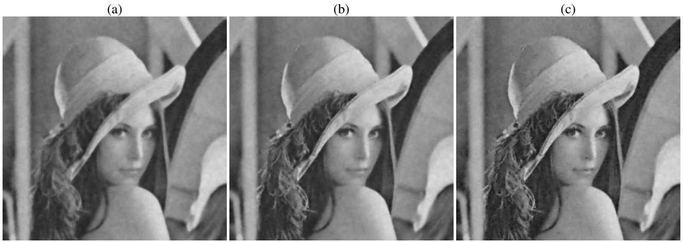
Fig. 2. Lenna: Restored images u by using (a) ITV, (b) ITV-TFR, and (c) NSAD-TFR model
